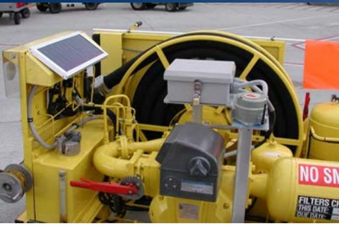
► *In order to supply constant power for the Varec Data Collection Units, a major airline installed a solar panel and gel battery cell to all stationary fueling carts as part of a fueling equipment improvement program.*
